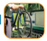
Lift the bicycle onto the rack, fitting the wheels into the slots labeled "Front" and "Rear". If the rack is empty, use the slot furthest from the bus.
