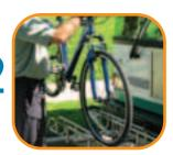
Lift the support arm and place it over the front tire, not on the frame or fender.
